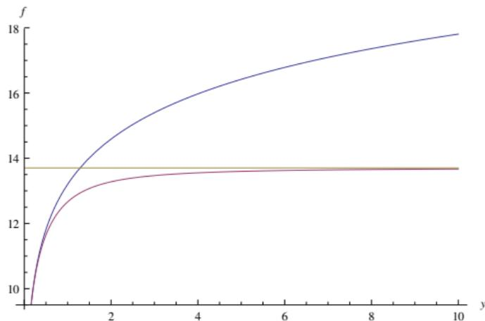
$\frac{1}{r} \gg T \gg m_D$ ,  $T \sim \frac{1}{r} \gg m_D$  and  $T \gg \frac{1}{r} \sim m_D$ . Discrepancy between blue and red lines signals a failure of color dipole approximation.
